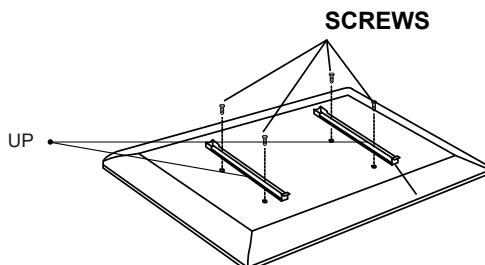
2. Identify the wall mount location and attach using the specified screws and anchors in the parts list. Drill holes to ensure the screws are securely attached to the wall.
