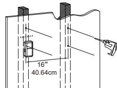
Use a 0.2" (5.5mm) drill bit to drill 2" (50mm) depth holes.
