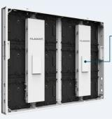
High heat-generating parts are integrated in the back box
