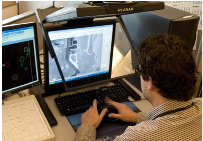
Picture 1: The StereoMirror design allows the space under the mirror to be utilized for keyboard or mouse.
