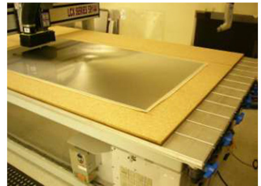
Fresnel and Image Screen on the cutting machine
