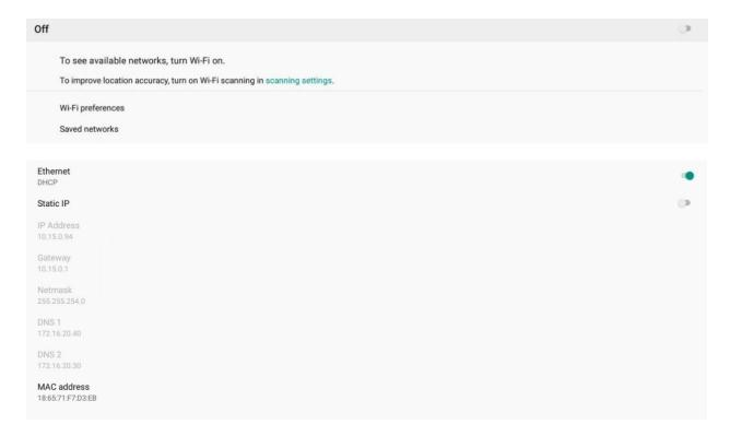
5. For Wi-Fi, select the desired network. For Ethernet, select Static IP to configure your IP settings. Press save when complete.
