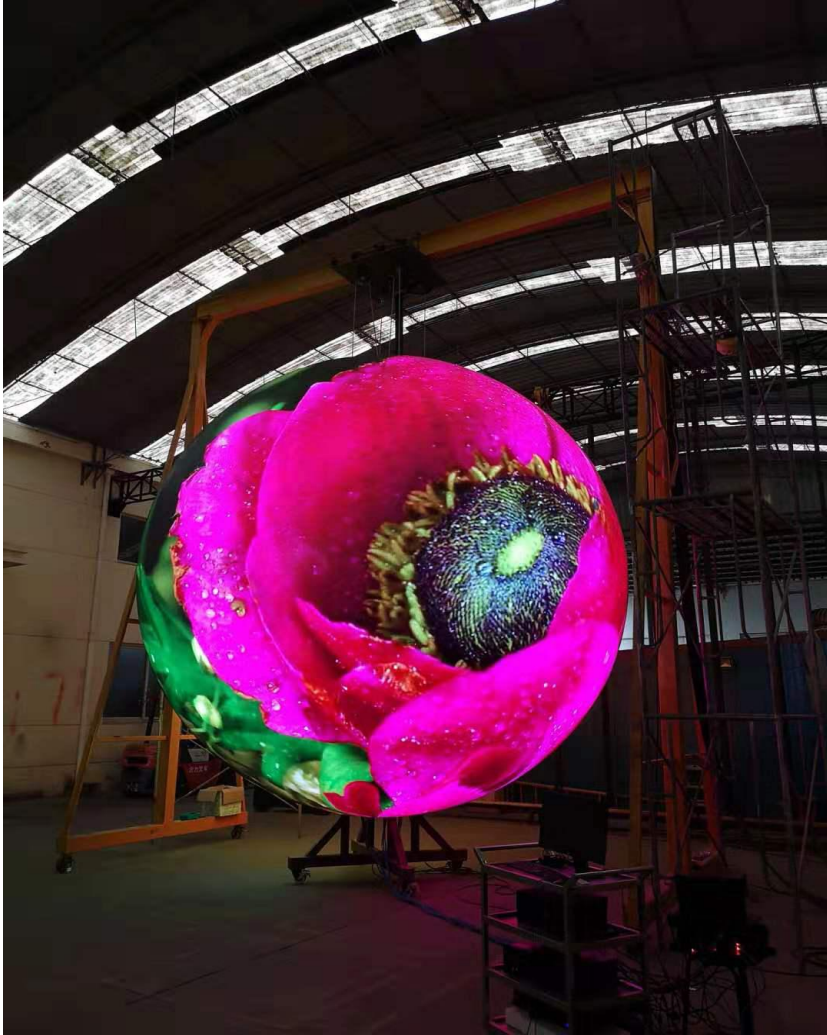
QUT-Indoor P3 LED Sphere with 5m Diameter and Mechanical up and down
