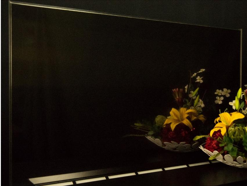
*Figure 8 - This image shows the back of a display (with a third-party lighting strip used to light the floral arrangement that is not part of the product). You can see the physical floral arrangement in the foreground and a reflection of that floral arrangement on the back of the screen without any content shown (full black or off).*
