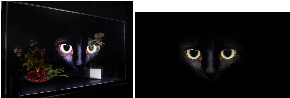
*Figure 2 - The same image on the transparent display on the left and the image to the right is the picture as it appears in Adobe® PhotoShop® or a photo editing program. This mostly black image as shown on a Planar LookThru Transparent OLED Display. Note: there is a small light strip behind this display that was put there to light the floral arrangements behind the screen. That is not part of the product itself.*
