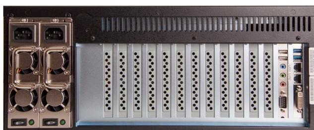
Clarity VCS features server-class CPU, 3rd generation PCIe switched fabric backplane, RAID solid state drives, redundant power supplies and modular expansion.
