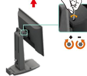
**Tension Torque Adjust**
