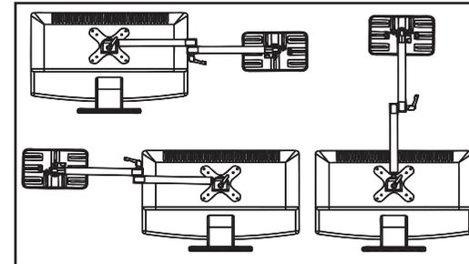
4. The mount can be adjusted to different positions.
