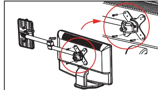
3. Install four screws to four corners VESA base.
