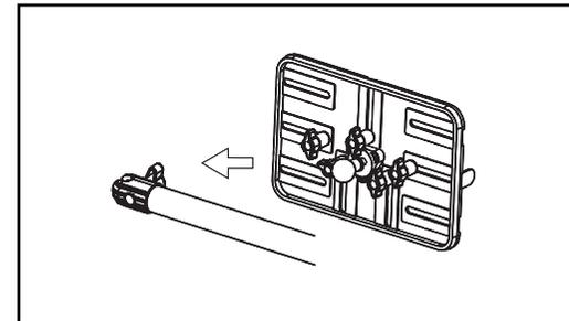
1. Screw L and ARROW CLIPS onto the TRAY with KNOBS. L Clips can be positioned (top/middle/bottom) to avoid buttons and connectors.
