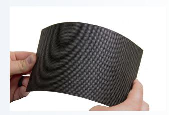
Planar® CarbonLight™ CLI Flex™ Series pliable LED video wall displays combine to create immersive and eye-catching concave or convex curved video walls. The LED modules are literally bendable, ideal for smoothly curved walls, waves, halos or column wraps. The modules can form curves as tight as 25″ or 637mm without color shift, offering a more visually-appealing alternative to faceting flat LED cabinets into segmented curves.
