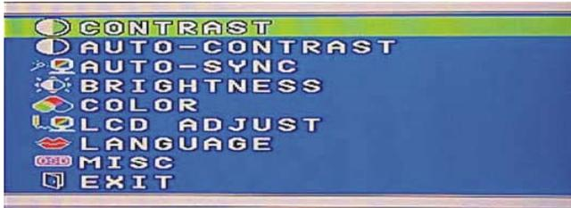
**CONTRAST** Adjusts the contrast level of the screen image. Under Main Menu, select CONTRAST using the [+] or [-] button, then press [Menu] button to activate the function. Press the [+] button to increase contrast, [-] button to decrease contrast shown below. Press [Menu] to return to Main Menu.
