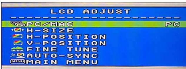
**PC/MAC** Switches between PC at 800X600 resolution and MAC at 832X624 resolution. Select PC/MAC, using [+] or [-] button. Then press [Menu] to initiate the switch between PC and MAC shown as above.
