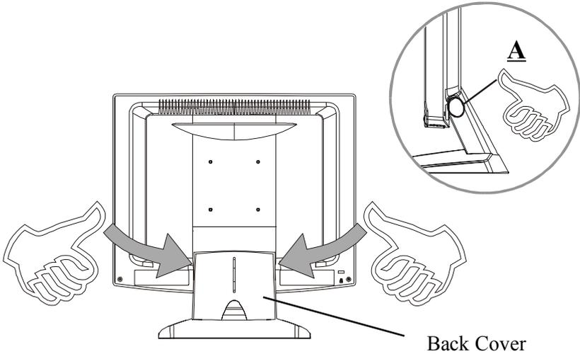
1. To remove the back cover, follow the arrows in Figure A and press with both your thumbs. The cover should be removed by pressing firmly.
