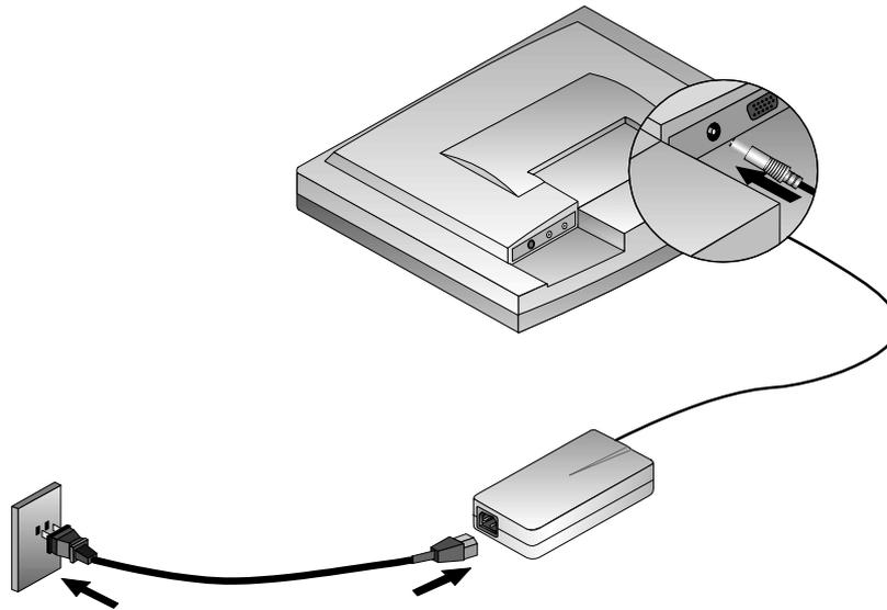
**Figure 1-5: Connecting Power to the LCD Monitor**
