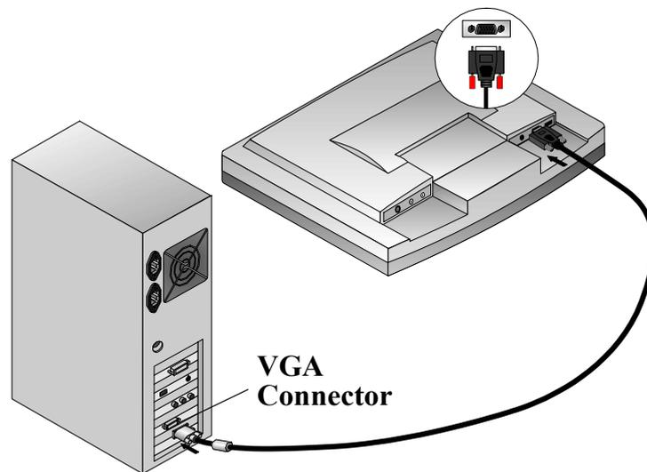
**Figure 1-6: Connecting the LCD Monitor to the PC**
