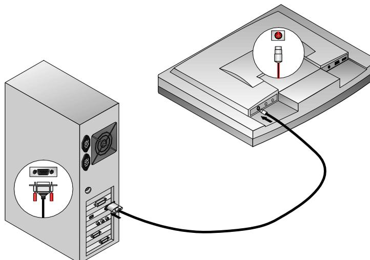
**Figure 1-8: Connecting the Optional Touch Screen Cable**
