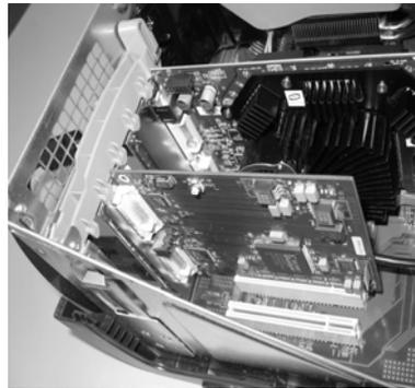
*Mirror-flip PCI card installed*
