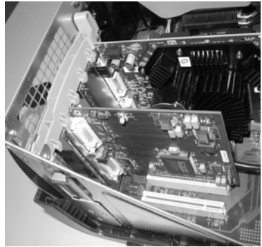
Mirror-flip PCI card installed.
