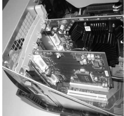
Figure 7. Mirror-flip PCI card installed.
