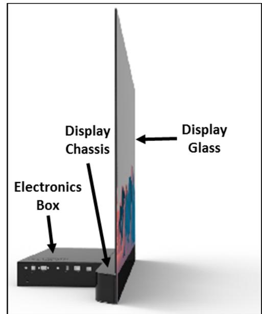
Note that the corners of the Display Chassis and the right side (viewed from the front) of the Electronics Box are chamfered at a 45° angle, allowing a corner or right-angle installation of Planar LookThru displays. This is a feature found in all the Planar LookThru displays. The bottom view of a Planar LookThru LO55 in the figure below illustrates the corner chamfers. The leveling feet and counterweight are also shown.
