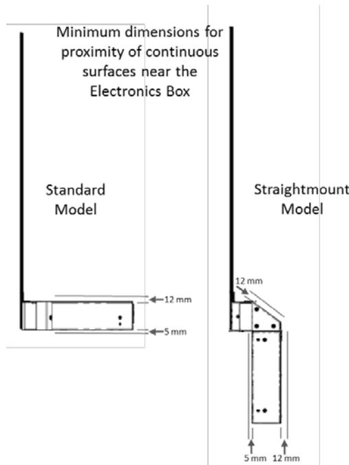
We do not recommend that either of the Straightmount Models be mounted where the weight of the display is carried by the bottom surface of the Electronics Box.
