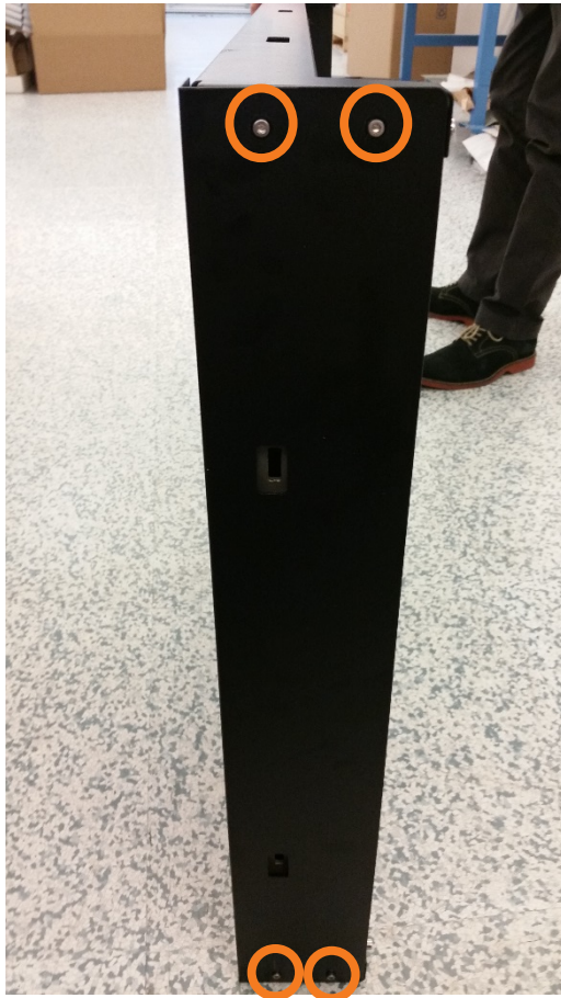
Figure 4. A side sheet metal protective cover is shown. Bolts are circled in orange.
