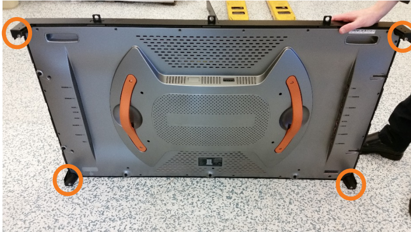
Figure 5. Top and bottom sheet metal protector bolts are circled in orange.
