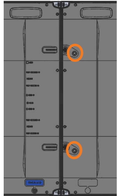
Figure 9. Use a 5mm hex key to tighten the two adjustment points.
