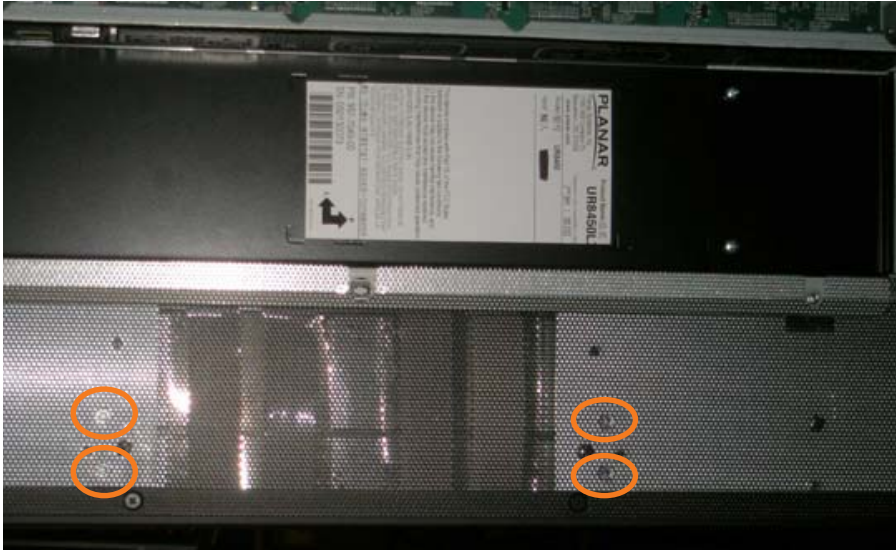
Landscape holes for kickstand bracket installation
