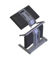
4. Thread the cables from the top monitor through the rectangular hole in the cross bracket.
