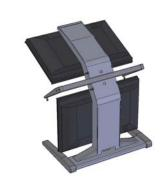
6. Remove the beamsplitter from the shipping case. With the StereoMirror™ logo oriented to the lower right, insert the pins located on either side of the mirror frame into the corresponding slots on the mirror support arms. The pins should rest in the fully forward position of the mounting arm slots.
