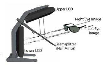
Operating principle of the StereoMirror monitor
