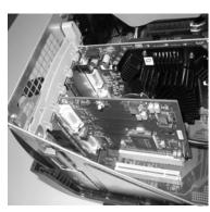
Mirror-flip PCI card installed
