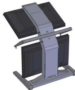
6. Remove the beamsplitter from the shipping case. With the StereoMirror™ logo oriented to the lower right, insert the pins located on either side of the mirror frame into the corresponding slots on the mirror support arms. The pins should rest in the fully forward position of the mounting arm slots.
