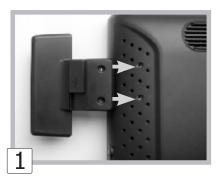
Place the MSR on the back of the monitor on the left side.
