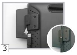
Connect the USB cable to the USB on the MSR.
