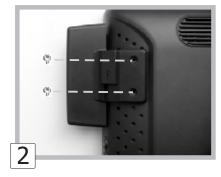
Secure the MSR to the monitor using the two screws provided.
