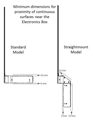
We do not recommend that the Straight Mount Model be mounted where the weight of the display is carried by the bottom surface of the electronic box.
