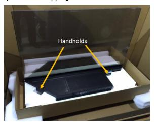
We recommend the display be handled by at least two people. At no time should the glass be held where the weight of the display is borne by the glass. Proper handling is demonstrated in the picture below.
