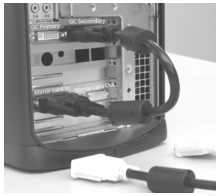
Figure 8. Short DVI cable installed.
